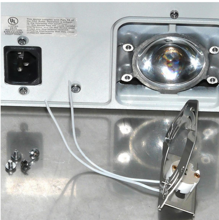
(2): Cut the lamp wires, and insulate the ends that are inside the microscope.
