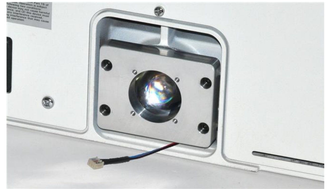
(4): Attach the adapter plate using the four M3 screws in the outer four holes. Secure with the 2.5mm hex key. Do not tighten one screw all the way, tighten each screw a little at a time so the O-ring is compressed evenly.
