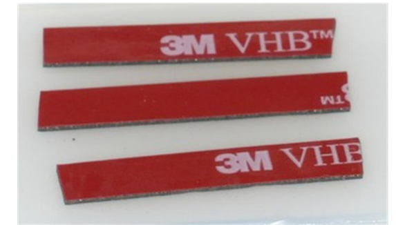
Tape to secure wires.
