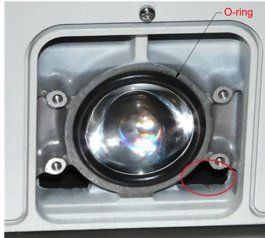
(3): Press the O-ring in place in front of the lens as shown. Feed the pot cable out through the hole circled in red above.
