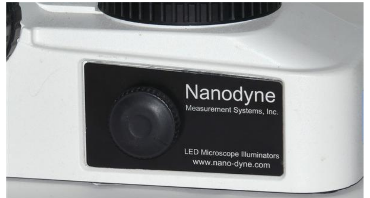
(6): Put the original knob on the new potentiometer shaft. Tighten with the 1.5mm hex key provided. For better appearance, back off the set screw so it fits on the round part of the shaft, rather than the flat, for a closer fit to the plate.
