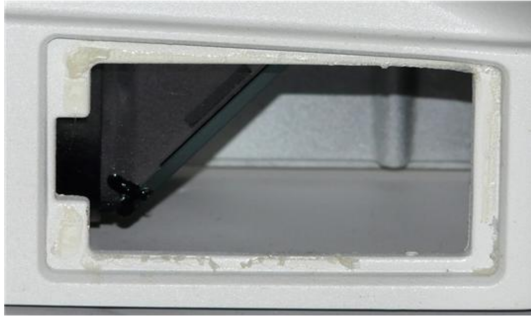
(1): Excessive glue residue left from the old plate. Remove before installing new plate.
