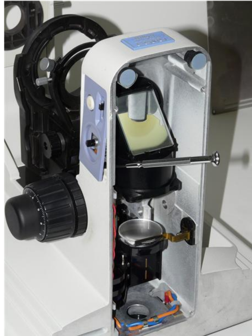
(2) Remove the original pot plate by pushing it out from the inside. Use a small screwdriver to pry if needed. Unplug it from the cable and discard.
