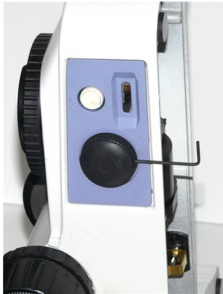
(1) Remove bottom cover (not shown). Remove and keep original adjustment pot knob. Remove using 1.5mm hex key.
